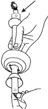
Thread the rod support (if previously removed or not present) so that it is positioned on the top flap (end three holes), then the top cap (2) and bottom cap (4); insert the electrical leads through the rod cavity. The wires should be inserted from the bottom upwards. Make sure no wires are on the outside.
