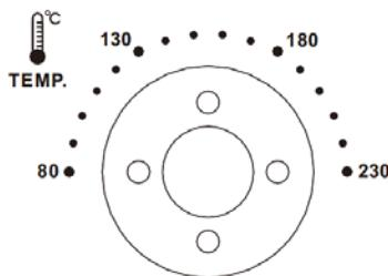
**Thermostat knob (1).** This sets the temperature inside the oven (max 230°C approx.): turn the knob to the temperature value required and the heating elements will switch on, switching off when the set temperature is reached, and back on again when it decreases.
