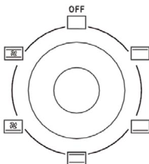
**Selector knob (2).** This selects the oven's cooking mode and operates the top and/or bottom heating elements or both.
